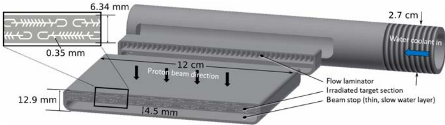
Figure V.41: Basic structure of the internally cooled target
