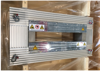
Figure VI.4: Prototype of the TFSM segment (left) and simulated and measured magnetization within the TFSM (left).
