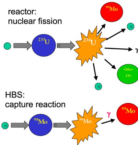
**Figure A.1:** Schematic of two possible routes to produce Mo-99, the parent nuclide of Tc-99m. Production in reactors by a fission reaction has a high cross section, but requires the use of nuclear fuel and leaves behind a significant amount of radioactive waste. Production by neutron capture at HBS has a lower cross section and results in less specific activity, but avoids the use of nuclear fuel material.
