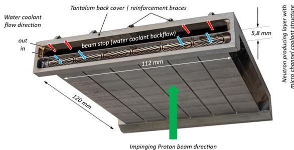
**Figure III.4:** Prototype of the 100 kW HBS target.
