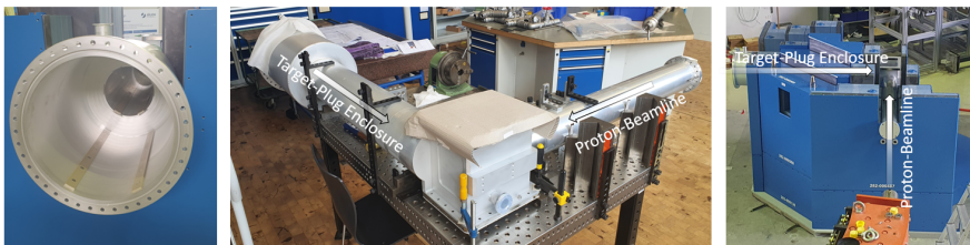
Figure II.22: left: look into the enclosure for the target plug of the L-tube; centre: L-tube (design of the 10 kW HBS prototype) which carries the target plug and continues the proton beam line; right side: L-tube inside partly build up target station prototype
