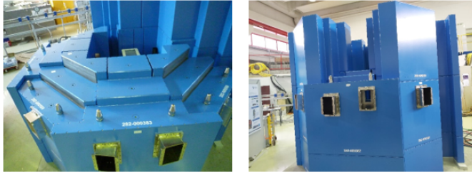
Figure A.9: iii) Assembly of the stationary part of the shielding
